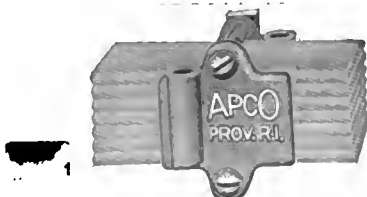
Apco spring leaf lubricator which uses felt pads
